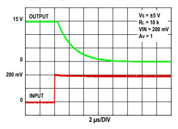
Figure 29. Positive Overload Recovery
