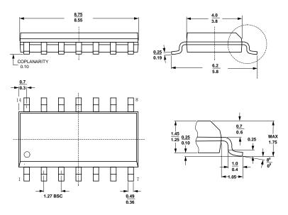
Figure 43. 14-Lead SOIC Package Dimensions shown in millimeters
