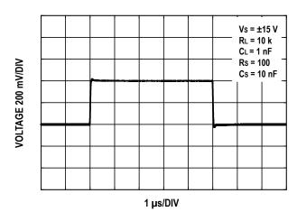
Figure 35. Capacitive Load Drive of 1 nF with Snubber
