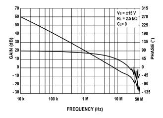
Figure 37. Frequency Response of Competitor JFET Amplifier
