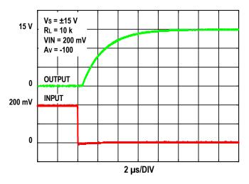
Figure 30. Negative Overload Recovery
