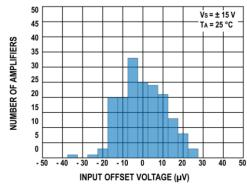
Figure 2. Offset voltage histogram
