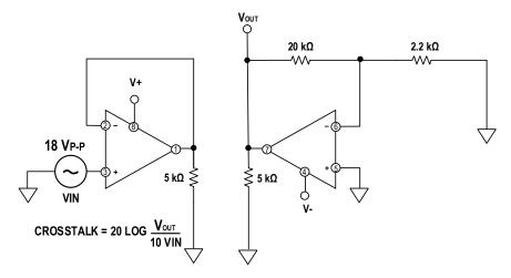
Figure 39. Crosstalk Test Circuit
