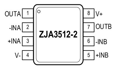
Figure 3. ZJA3512-2 Pin Configuration (8-lead SOIC and MSOP)
