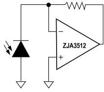
Figure 1. Photodiode amplifier
