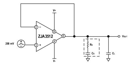
Figure 31. Snubber Network Configuration
