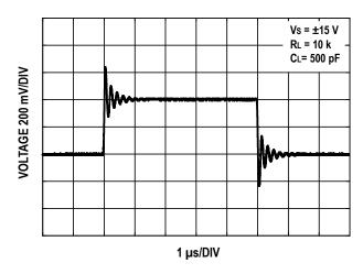
Figure 32. ZJA3512 Directly Driving Large Capacitive Load
