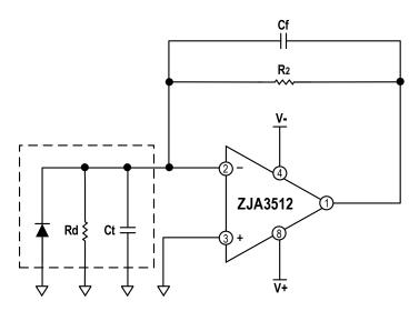
Figure 38. Equivalent Preamplifier Photodiode Circuit
