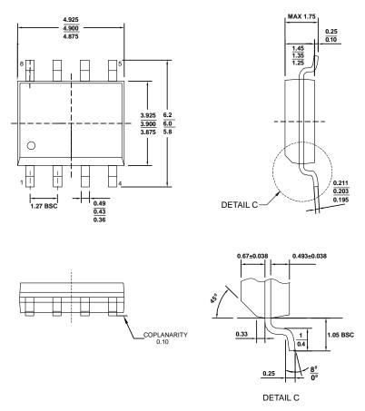
Figure 41. 8-Lead SOIC Package Dimensions shown in millimeters
