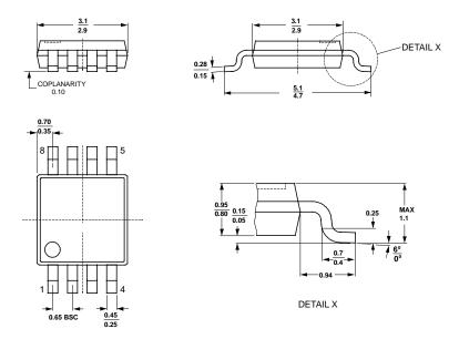
Figure 42. 8-Lead MSOP Package Dimensions shown in millimeters
