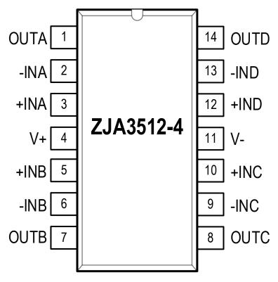
Figure 4. ZJA3512-4 Pin Configuration (14-lead SOIC)
