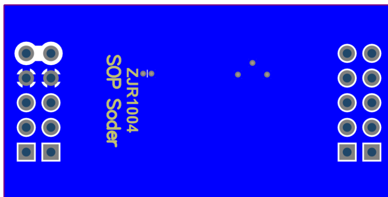
Figure 20. ZJR1004 Evaluation Board Layout (Bottom Layer)
