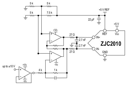
Figure 31. Realizing Bipolar Single-Ended Conversion to Fully Differential via Dual Op Amps
