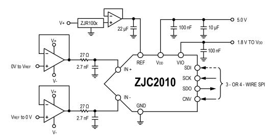
Figure 27. Application Circuits Using Multiple Power Supplies
