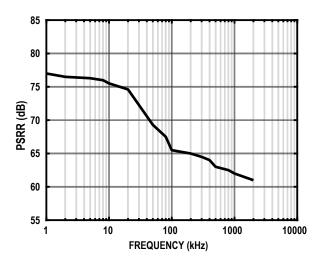
Figure 36. PSRR vs. Frequency
