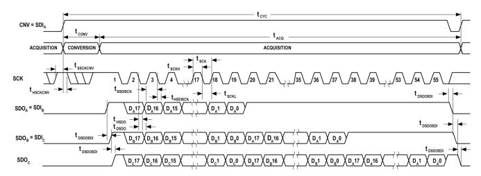
Figure 49. Chain Mode (with Busy Indication) Serial Interface Timing
