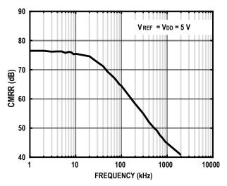
Figure 29. Analog Input CMRR vs. Frequency
