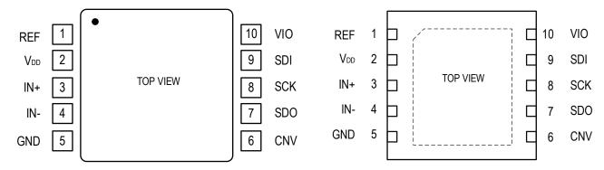
Figure 3. 10-lead MSOP pin configuration
