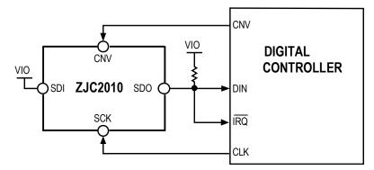
Figure 40. Chip select mode (three-wire type with busy indication) connection diagram
