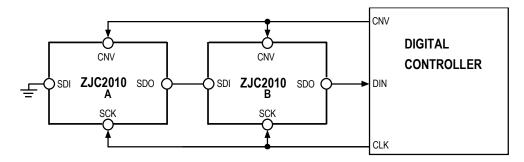
Figure 46. Chain Mode (without Busy Indication) Connection Diagram
