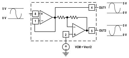
Figure 32. High Input Impedance Unipolar Single-Ended to Fully Differential
