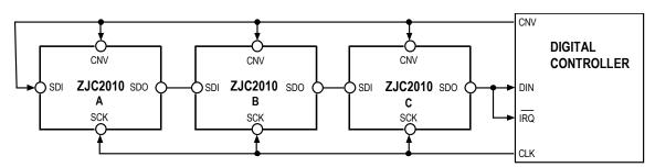
Figure 48. Chain Mode (with Busy Indication) Connection Diagram
