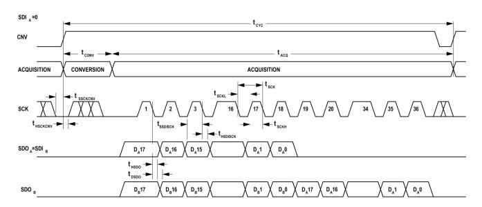
Figure 47. Chain Mode (without Busy Indication) Serial Interface Timing
