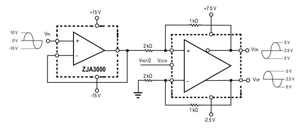
Figure 34. High Input Impedance Bipolar Single-ended to Fully Differential
