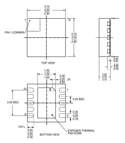
Figure 52. 10-Lead DFN Package Dimensions Shown in Millimeter
