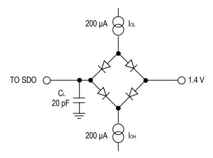
Figure 5. Load Circuit for Digital Interface Timing
