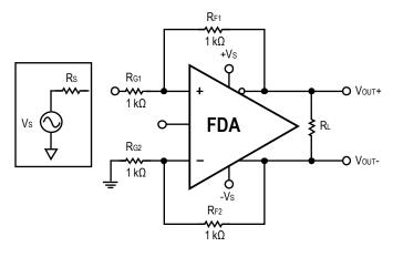
Figure 33. Realizing Bipolar Single-Ended to Fully Differential via Differential Op Amp
