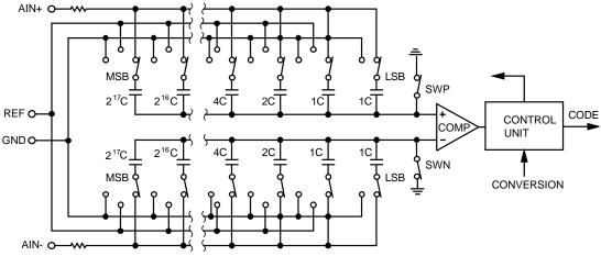
Figure 25. ADC Simplified Circuit Diagram
