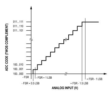
Figure 26. ADC Ideal Transfer Function
