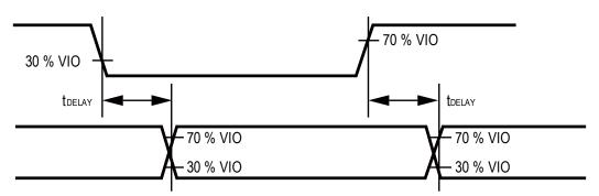
Figure 6. Voltage Levels for Timing
