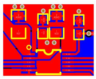
Figure 50. Example Layout and Routing of ZJC2010
