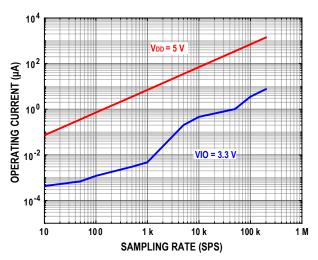
Figure 37. Operating Current vs. Sampling Rate
