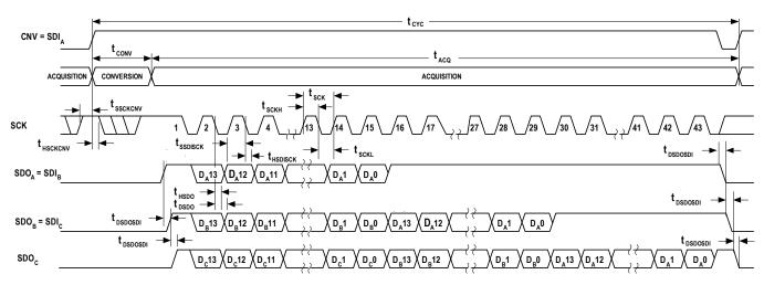
Figure 47. Chain Mode (with Busy Indication) Serial Interface Timing
