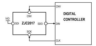
Figure 36. CS Mode (3-wire without Busy Indication) Connection Diagram
