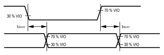
Figure 6. Voltage Levels for Timing
