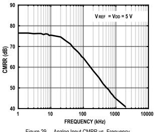
Figure 29. Analog Input CMRR vs. Frequency
