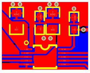
Figure 48. Example Layout and Routing of ZJC2017
