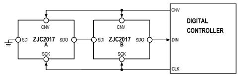
Figure 44. Chain Mode (without Busy Indication) Connection Diagram
