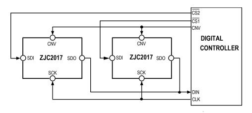
Figure 40. CS Mode (4-wire without Busy Indication) Connection Diagram
