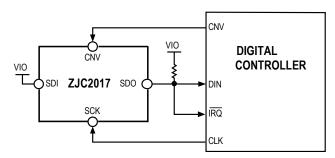
Figure 38. Chip Select Mode (three-wire type with busy indication) Connection Diagram
