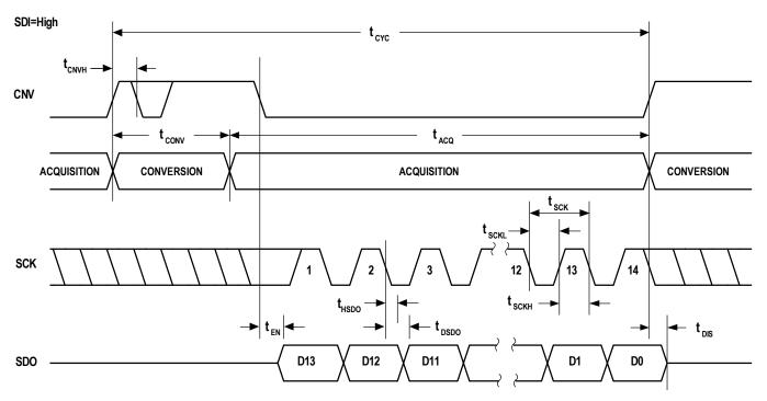
Figure 37. CS Mode (3-Wire without Busy Indication) Serial Interface Timing
