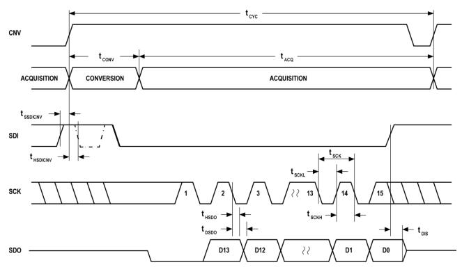
Figure 43. CS Mode (4-wire with Busy Indication) Serial Interface Timing
