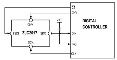
Figure 42. CS Mode (4-Wire with Busy Indication) Connection Diagram
