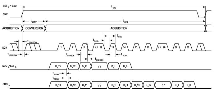
Figure 45. Chain Mode (without Busy Indication) Serial Interface Timing
