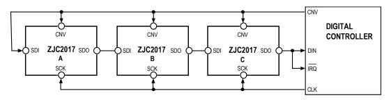
Figure 46. Chain Mode (with Busy Indication) Connection Diagram
