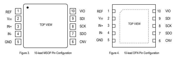
Note: The exposed pad has no internal connection. Connect the pad to GND.
