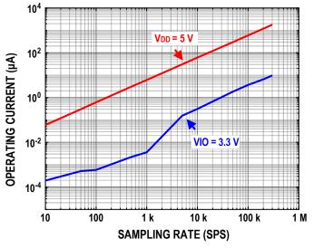
Figure 35. Operating Current vs. Sampling Rate
