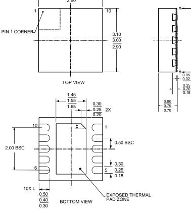
Figure 50. 10-Lead DFN Package Dimensions Shown in Millimeter
