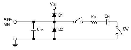
Figure 28. Two Diodes D1 and D2 Provide ESD Protection for the Analog Inputs
