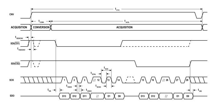
Figure 41. CS Mode (4-Wire without Busy Indication) Serial Interface Timing
