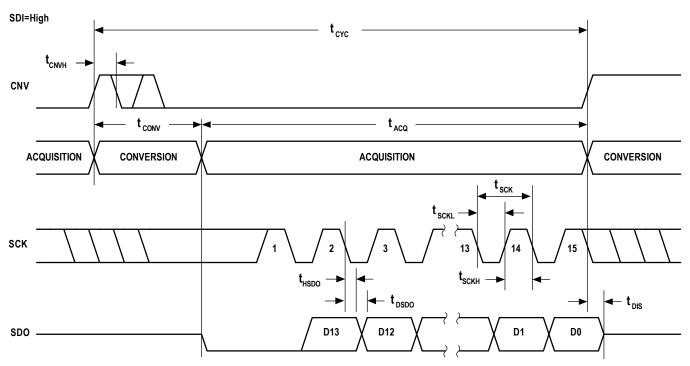
Figure 39. CS Mode (3-Wire with Busy Indication) Serial Interface Timing
